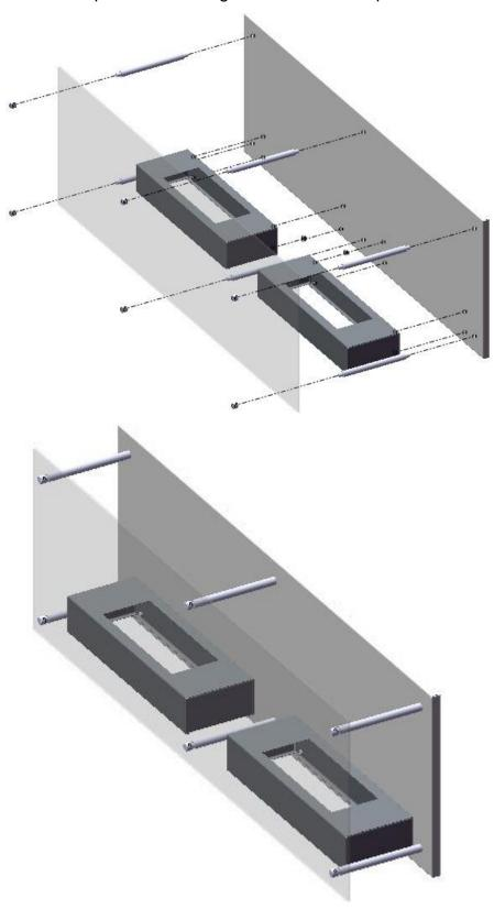
2. Mount the mounting bar unit to the wall using screws, and wall plugs.
