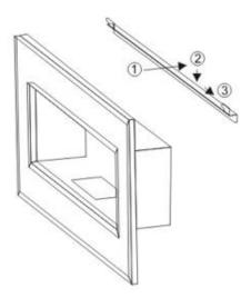
4. Place the burner into the burning chamber of the fireplace body.
