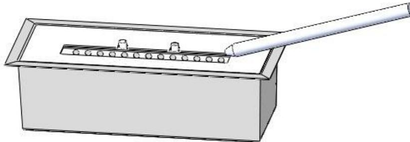
**CAUTION:** Fuel will burn low at first. Please allow 15 minutes to reach the optimum temperature and flame height. Opening or closing the sliding cover on the burner with the puller can adjust the flame.
