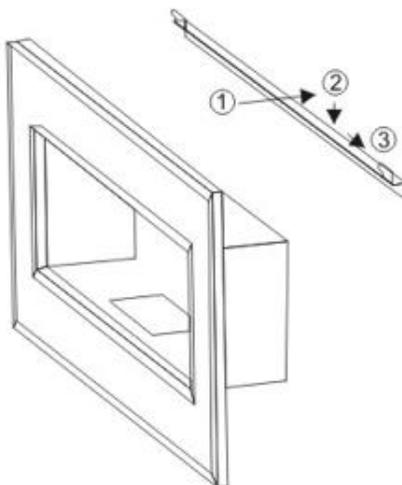
3. Place the burner into the burning chamber of the fireplace body.
