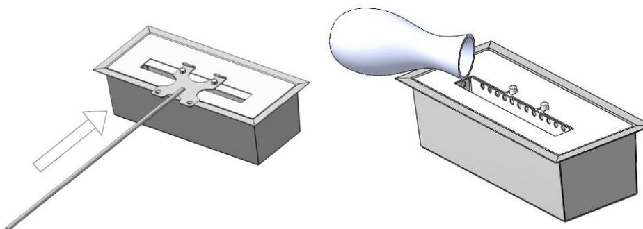
**Caution:** Spilled ethanol must be removed with an absorbent tissue and cleaned with water to prevent ignition outside the burner reservoir.
